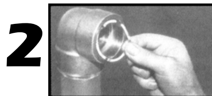
Fitter seats ring into fitting. Spring tension holds ring tightly in place, assuring no rattling or vibration even under extreme pressure Ring actually be-
